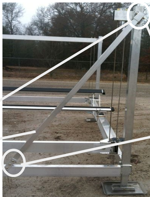
Diagonal Support Connection View on assembled hoist
