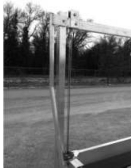
Non Winch Column front corner shown with Stabilizer Tube attachment.
