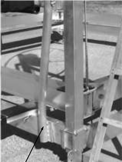
Diagonal Support/Stabilizer Tube Connection on Winch Column. Wheel shown will be attached in a later step.
