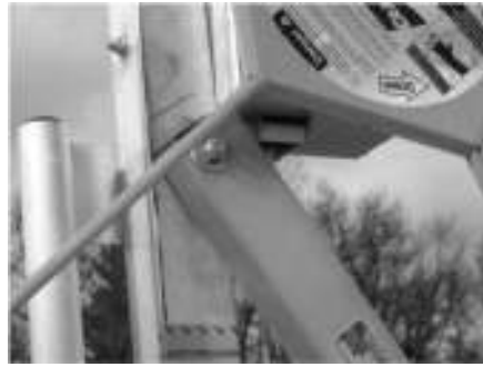
Diagonal Support/Stabilizer Tube Connection on Winch Column. Wheel shown will be attached in a later step.
