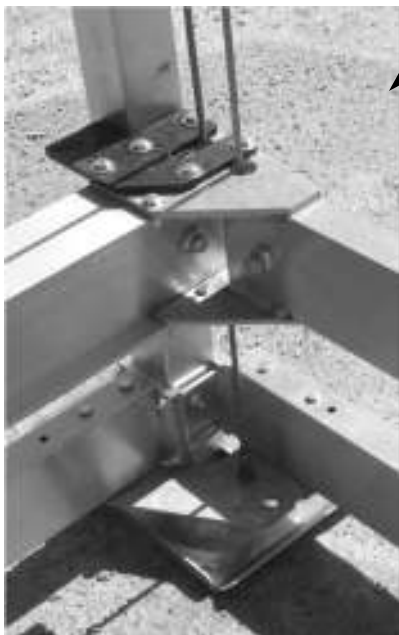
Winch column opposite area assembled view
