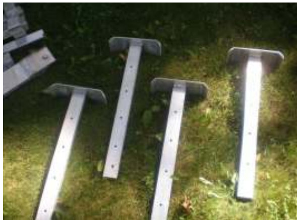
Four V1684 welded legs
