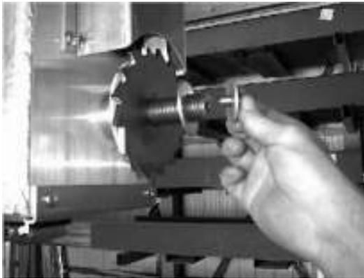
Next, take the 3/8" x 1" bolt out of the winch threaded shaft and steel washer. As shown above.
