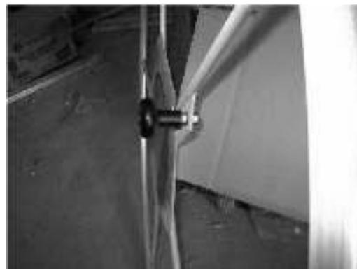
The wheel is missing the knob yet. Find a 3/8" x 2 1/2" bolt and 2- 3/8" whiz nuts. Put the bolt through the knob and spin one of the whiz nuts on. Don't spin the nut all the way to the knob or else it won't turn freely, leave a small gap. Put the rest of the bolt through the hole in the wheel plate and put a nut on the back side. Use a open end 9/16" wrench to hold the nut by the knob and tighten the nut on the back side of wheel plate.
