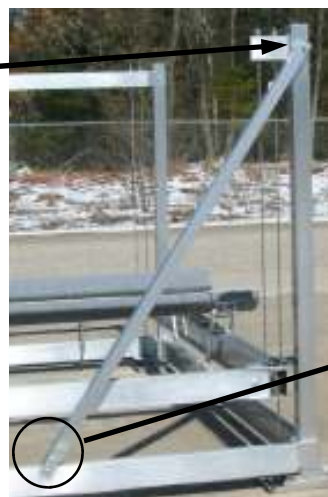
View of 3/16 x 2 x 6" long flat bar (4-req'd) on diagonal braces secured with 3/8 x 2 3/4 hex bolts and 3/8 whiz nuts. (6-req'd)
