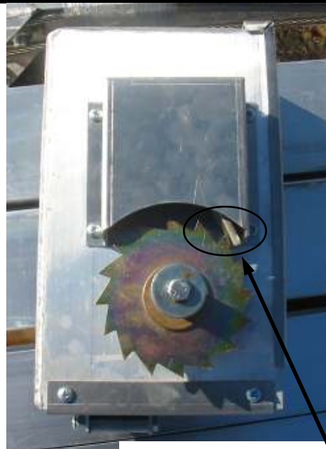
Ratchet, never lift up as this will cause uncontrollable spin
