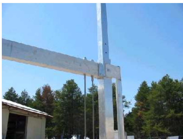
View of upper tube kitty corner to winch side showing cable with lock nuts and washers.
