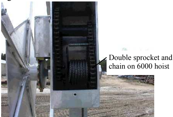
Winch bolted to hoist with wheel assembled. Cable goes through bottom of winch.
