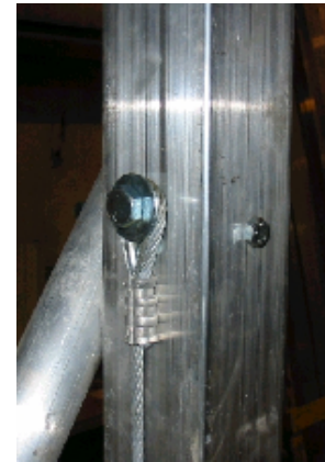
13.) Raise looped cable end and attach to winch column with 1/2" x 4 1/2" bolt, nut and washer.
